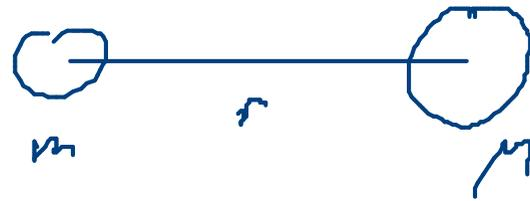
$$\left[ \begin{array}{l} \Rightarrow \\ \text{z.B.} \end{array} m \frac{v^2}{r} = \gamma \frac{mM}{r^2} \Rightarrow M = \frac{v^2 r}{\gamma} \right]$$
